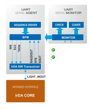
**Figure 1: Verifying an SoC UART interface with the UART** *e***VC** The Serial Agent is used to drive frames into the UART interface. The Monitor is used to check bidirectional communication and score board data on both the transmit and receive paths (not shown here).
